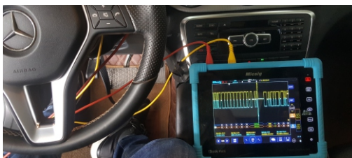
Power CAN bus communication
