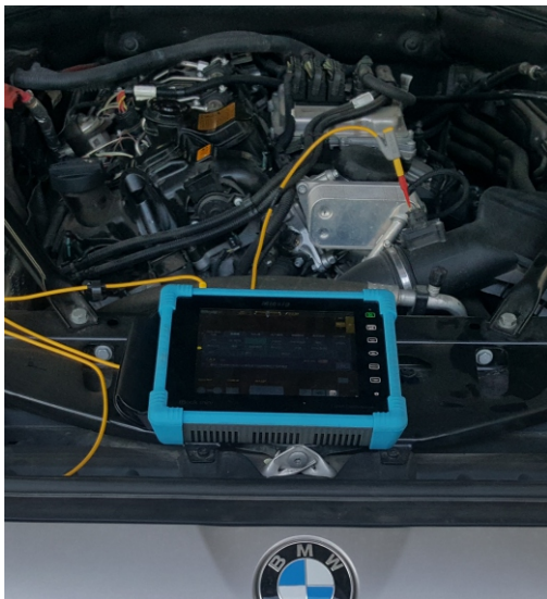
BMW Air flow meter test
