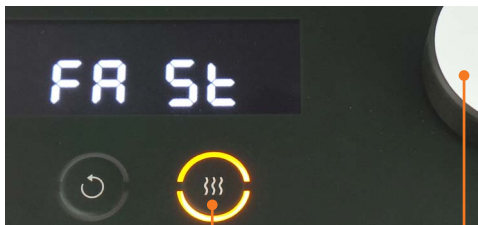
Heating button: blinking
