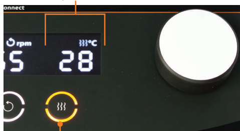
Heating button: Heating on
