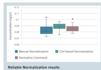
Normalization of human gDNA present in a 96-well plate at 8 concentrations in triplicates (24 wells) to a target value of 0,1 ng/ $\mu$ l. Measurement of the gDNA concentrations in the destination plate by fluorometric quantification.
