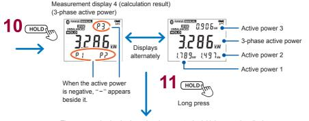
The measured value is cleared and returns to the initial connection display.
