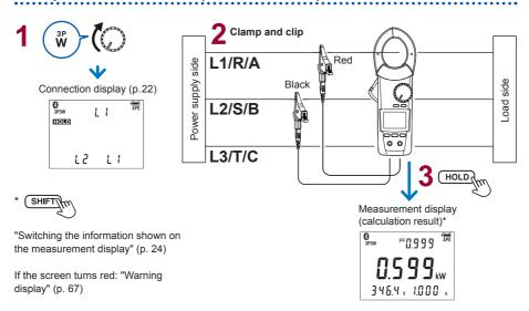
When the balanced 3-phase 3-wire zero-cross phase angle is less than -90° or exceeds 90°, the measured value appears "----".
