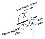
Align the current direction mark with the direction of the current.
