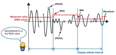
AVG: Average value after pressing the MAX/MIN key MAX: Maximum value after pressing the MAX/MIN key
