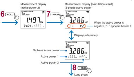
The measured value is cleared and returns to the initial connection display.
