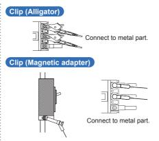
(If unable to connect the magnetic adapter so that it sits perpendicular to the terminal due to the weight of the voltage cord, connect it at an angle so as to balance it against the weight of the cord.)
