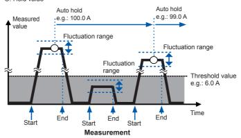
If the measured value\* (voltage, current, or active power) falls below the threshold value once and the two conditions are satisfied again after automatic retaining, the measured value at that point will retain automatically.
