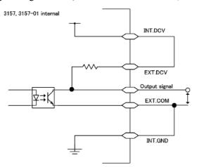
2. When using the external power supply
