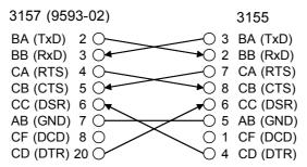
Specification: D-subminiature 25-pin male to D-subminiature 9-pin female connectors, with "crossed" data connections
