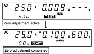
Zero adjustment is possible within a range equivalent to a resistance between 0.000  $\Omega$  and 0.100  $\Omega$ , on either the voltage or resistance indicator. If the measured value falls outside this range, either the resistance value or the voltage value will blink, and the unit will enter READY state.
