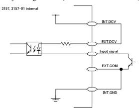
2. When using the external power supply
