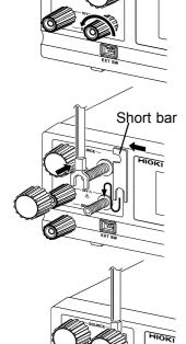
(2) Connect the probe and short bar as shown in the figure on the left.
