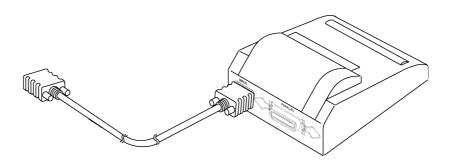
Use the 9442 PRINTER, the 9443\* AC ADAPTER, and the 1196 RECORDING PAPER. To connect the main unit and printer, use the 9593-02 RS-232C INTERFACE and the 9446 CONNECTION CABLE. (All are options.)
