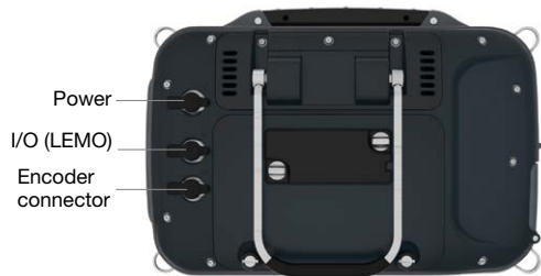
Connector ports, back panel
