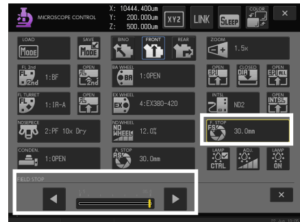
[F. STOP] button, sub screen: DIA field diaphragm adjustment
