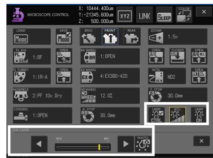
[LAMP CTRL] button: Switch lamp control Sub screen: Brightness adjustment operation
