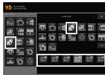
DS-L3 [MICROSCOPE CONTROL] screen control button configuration (Example of specifying Epi-fluorescence cube turret → Filter cube)
