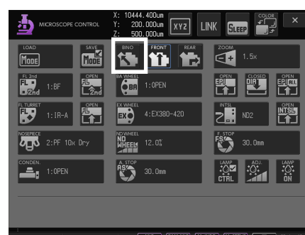
[BINO] button: Binocular optical path 100%
