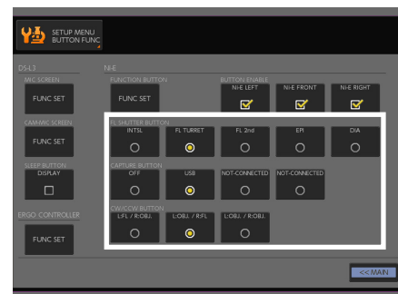
Function setting of FL SHUTTER, CAPTURE, and CW/CCW buttons
