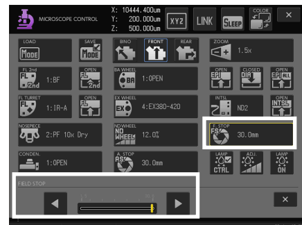
[F. STOP] button, sub screen: DIA field diaphragm open
