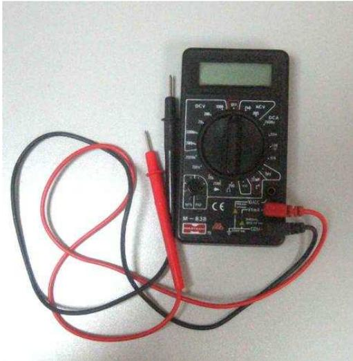
A photograph of a digital multimeter, model M-838, lying on a light-colored surface. The multimeter is black with a digital display at the top. It has a rotary selector dial in the center and several buttons on the right side. Two test leads are connected to the device: a red lead with a pointed tip and a black lead with a pointed tip. The leads are coiled around the multimeter. |
