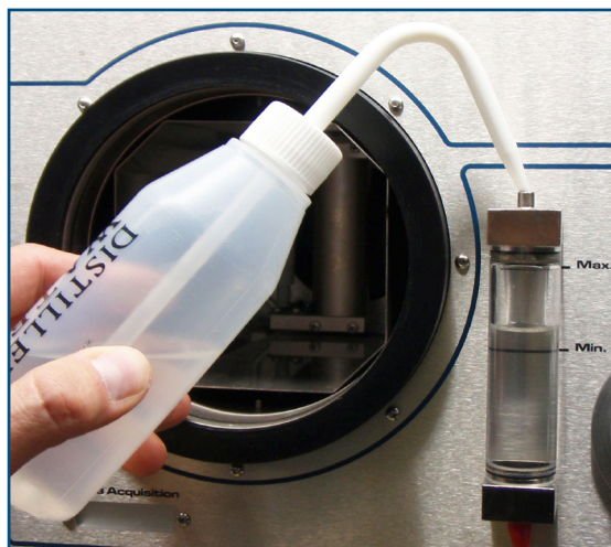
Figure 5 Filling the Water Reservoir
