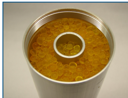
Figure 8 Level of Silica Gel Required
