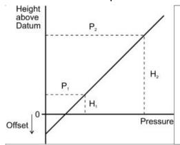
The relationship between pressure and depth in shallow water is a straight-line function:
