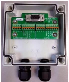
The bare cable from the VRS-20 should be passed through the cable gland and terminated in the push fit connectors with reference to the wiring schedule.
