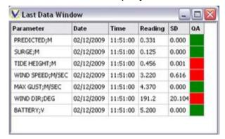
This data display mode allows the most recent reading from multiple sensors to be displayed in a tabular format.
