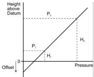
The aim of a site calibration is to derive a suitable gain and offset value by measuring the relationship between pressure and tide at the top and bottom of the tidal range.
