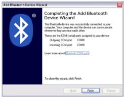
At this point you will be assigned two COM port numbers, the important one is the outgoing COM port as you will need to select this port when connecting to the instrument.
