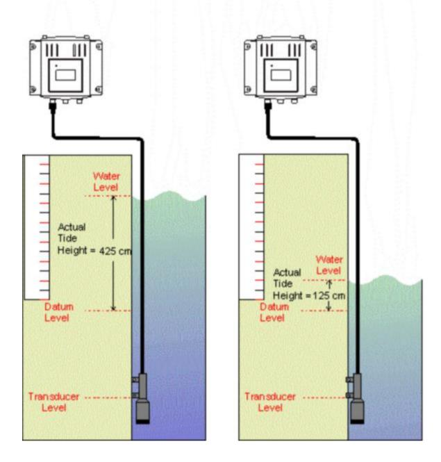
Install and fix the transducer in the desired position, and connect it to the TideMaster Run the TideMaster Express program on the PC.
