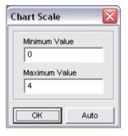
The Y axis of the graph will auto-scale for each parameter, to cover the range of data currently being displayed. The resolution of the axis labels may therefore change over time. It is possible to fix the range of each axis by right-clicking the axis. This will display this dialogue box:
