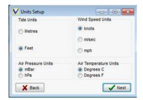
Data is both logged and output in the selected format. For a pressure sensor the conversion from pressure to depth will be based on the calibration factors stored in the TideMaster. This is not required for a radar sensor.
