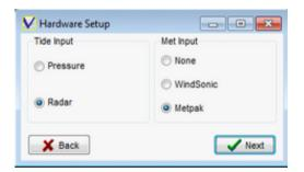
The fitted sensors can be enabled/disabled
