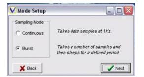
Battery lifetime requirements are critical to the choice of sampling pattern and further consideration to projected battery lifetimes are given in **section 3.4**
