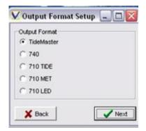
Real time output can be transmitted in a number of formats. The choice of format does not affect the logged data which is always stored in the same format.
