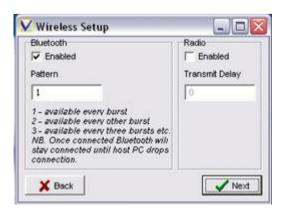
All TideMasters are fitted with Bluetooth for short range serial communications. If not required then this should be disabled as it uses up valuable battery capacity. To retain Bluetooth and save power it is possible to reduce the number of bursts the Bluetooth is made available for.
