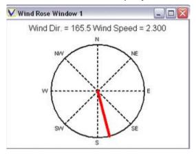
The wind rose display provides a convenient indication of the direction from which the wind is currently blowing, as well as giving a numerical indication of the magnitude and bearing.
