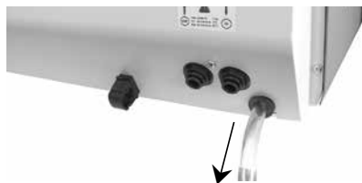
2 Place drain hose in laboratory drain
