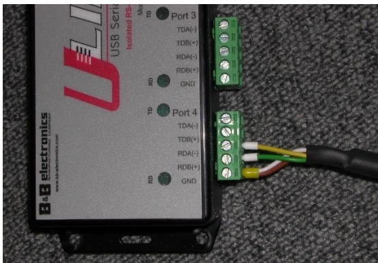
Figure 13 RS485 connection to transducer.
