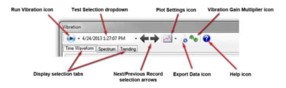
Figure 79. Vibration window controls.
