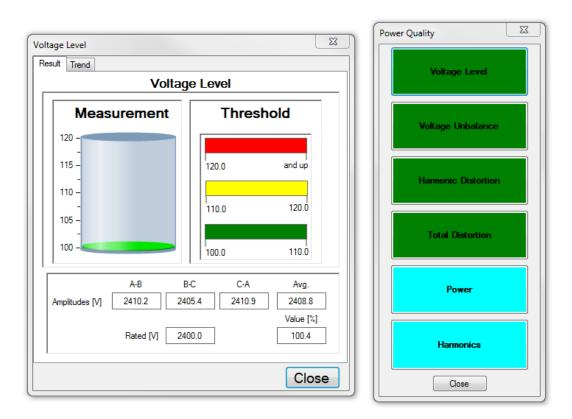
Figure 9. Voltage level test within the Power Quality domain.
