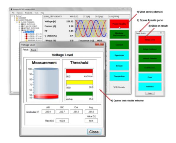
Figure 2. Selecting test results to display using Results panels.
