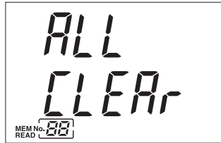
ALL CLEAR alarm indication
