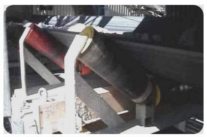
Figure 11 - 1. Conveyor Idler Rollers.
