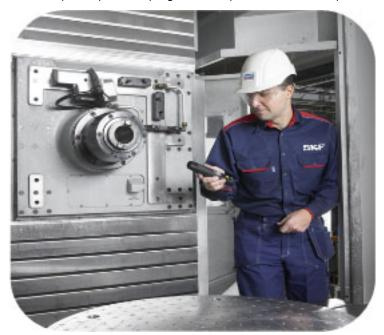
Figure 10 – 30. Monitor the Speed with a Tachometer.
