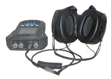
Figure C - 1. Headphones Connected to GX Series Microlog.
