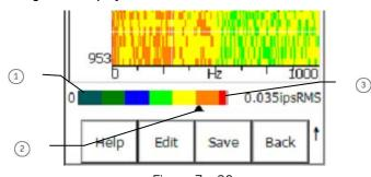
Figure 7 - 28. Spectrogram "Display Status" Indicators.
