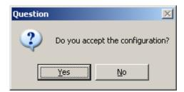
If accepted, the *network scan* window will close and the *PROFIBUS Master Configuration* window will be populated with the slaves that were found during the network scan.
