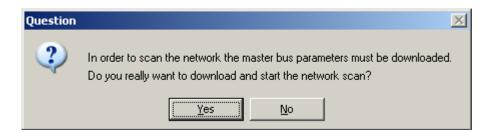
When the download is completed, the *PROFIBUS Master Configuration* window will initialize the Master to operate as a *Class 2 Master only*. In this mode it is possible to initialize the Master even if the database does not contain any slaves. After successful initialization, the *PROFIBUS Master Configuration* window will issue the following mailboxes in order to gather information about the connected slaves:
