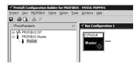
5 Double-click the **PROFIBUS MASTER** icon in the *Bus Configuration* window. This action opens the *Master Properties* dialog box.
