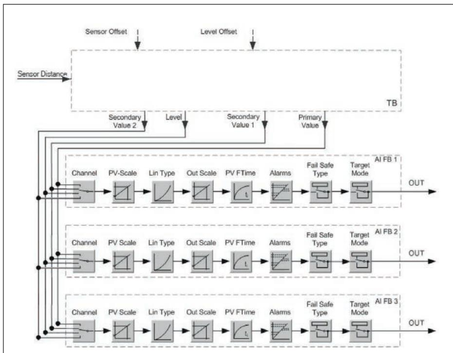
Рис. 55: VEGAFLEX 83: Block diagram with AI FB 1 ... AI FB 3 OUT values
