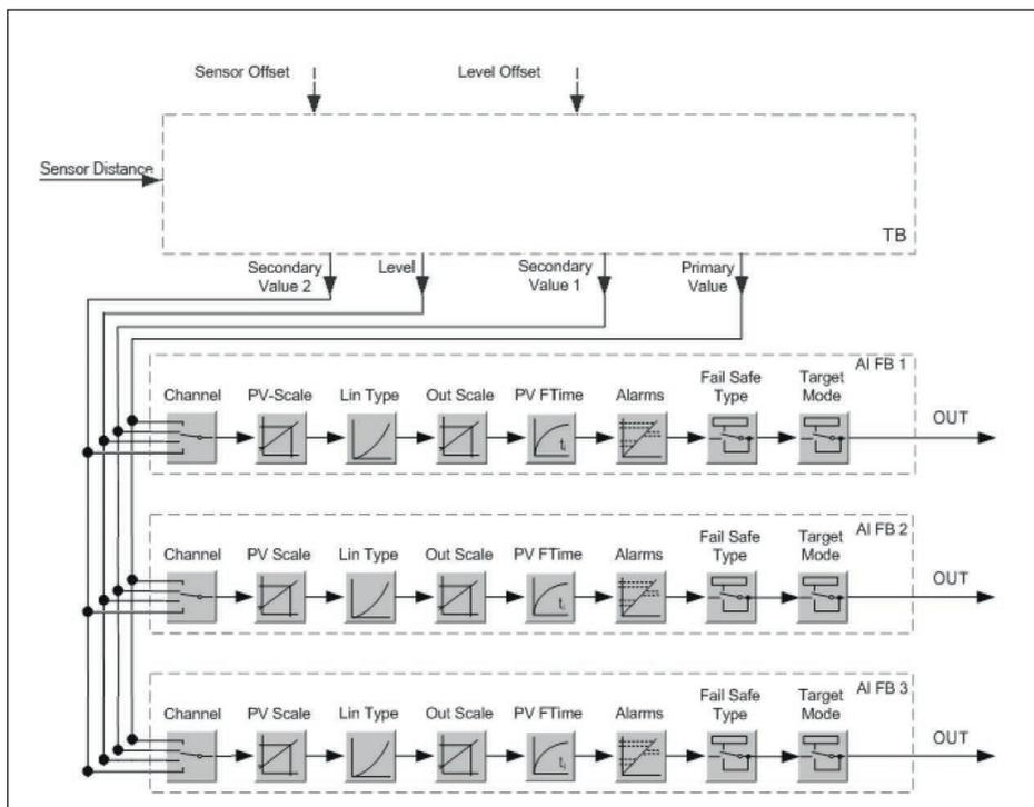
Рис. 60: VEGAPULS 62: Block diagram with AI FB 1 ... AI FB 3 OUT values
