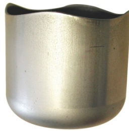
Deep Drawing Cup Test
