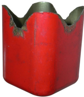
Square Deep Drawing Cup Test
