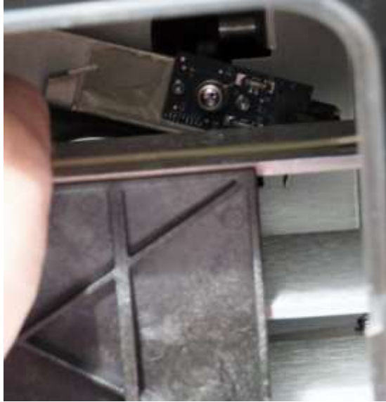
Figure 13 Sensor Probe Location
