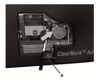
**8.** Slightly raise the injector (A) to remove it from the catch.
