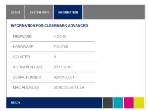
Information about the ClearMark Advanced is displayed here, e.g. which firmware version is currently in use or how many Marker Cards have been printed.
