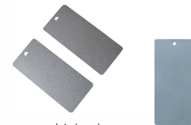
spray sand steel panels Phosphated steel panels
