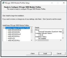
The default location of the installed module profile is C:\Program Files (x86)\Rockwell Software\RSLogix 5000\Module Profiles\RA 432ES GL-EIP.
