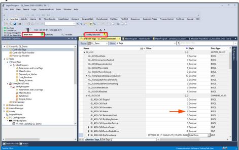
A simple program is created to monitor each node. If a safety demand is placed on a node, the node trips and its Pt.Data tag sets to 1. In <u>Figure 49 on page 51</u>, The MainProgram tab shows that a safety demand is placed on the Black node (Node 0), while all other nodes have no safety demand.
