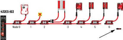
2. Remove the terminator from node 6 (see <u>Figure 70</u>).
