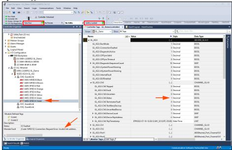
The following recommended steps show how to add nodes to a channel. You can perform these steps with power applied to the 432ES-IG3 network interface module.
