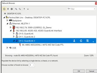
The window populates with all devices on the selected channel, along with the address and firmware in each device. In <u>Figure 19 on page 29</u>, there is only one device on channel 0.
