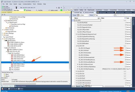
To correct this error, first delete the node, and add the correct catalog number.
