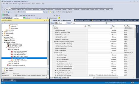
Before you insert the node at position 4 in the Controller Organizer, you must reassign the current nodes Yellow (4) and Green (5) to positions 5 and 6. This change preserves any logic or automatic diagnostic reporting that is associated with nodes 4 and 5 because the logic is associated with the node name, not the node number.
