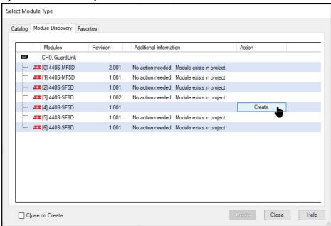
As shown in <u>Figure 65 on page 60</u>, the node number automatically assigns to the first open position, which is position 4.
