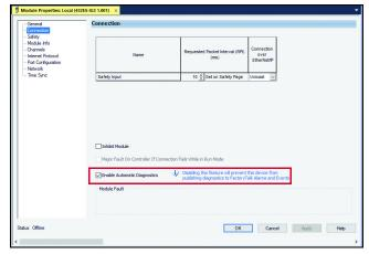
Only device Add-on Profiles (AOP) that have been updated with additional diagnostics show the Enable Automatic Diagnostics checkbox (<u>Figure 90</u>). You can use this checkbox to verify if the AOP of your device has been updated with additional diagnostics.
