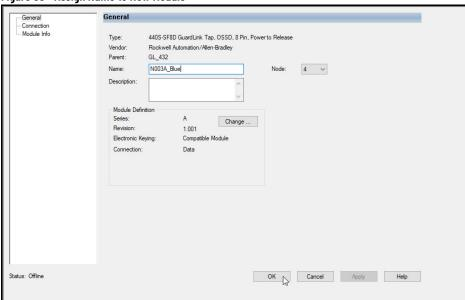
11. The Blue node appears in position 4. You can now add code to the Main Routine to capture the event when the Blue node trips, see <u>Figure 56 on page 55</u>.
