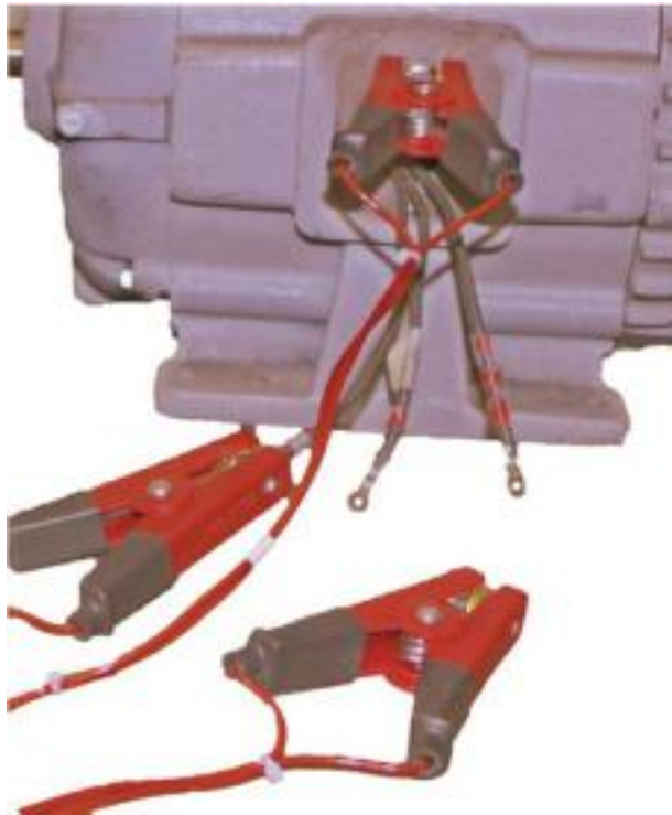
Figure 80. Capacitance test lead connections.
