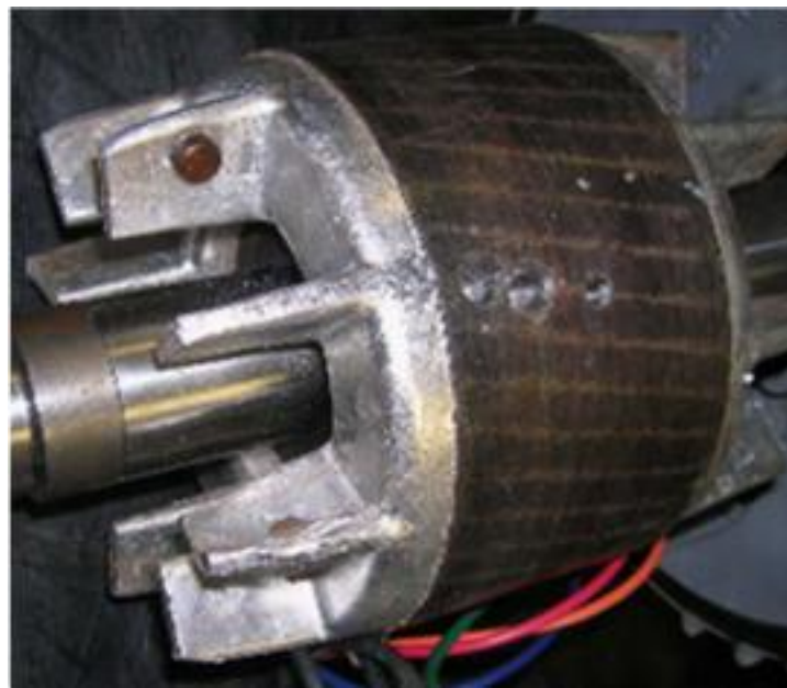
Figure 201. Delco 3hp showing rotor bars drilled completely through
