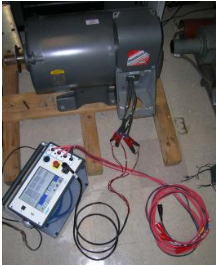
Figure 69. Connect RLC test leads to motor leads.
