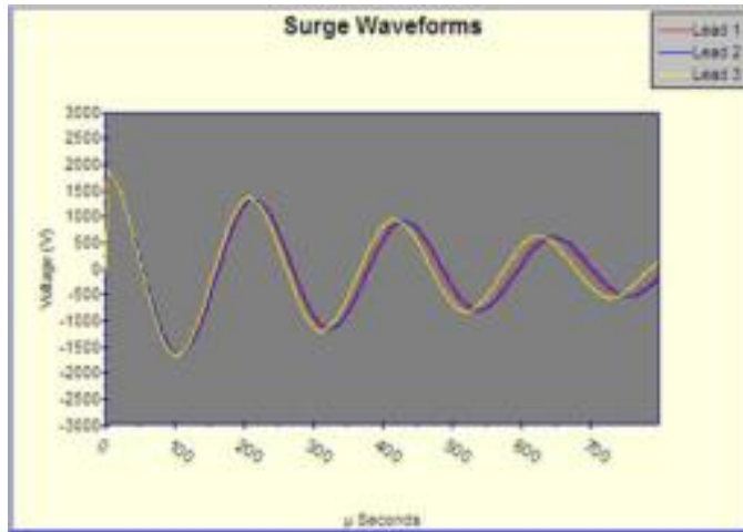
Figure 219. Surge waveform showing rotor coupling.
