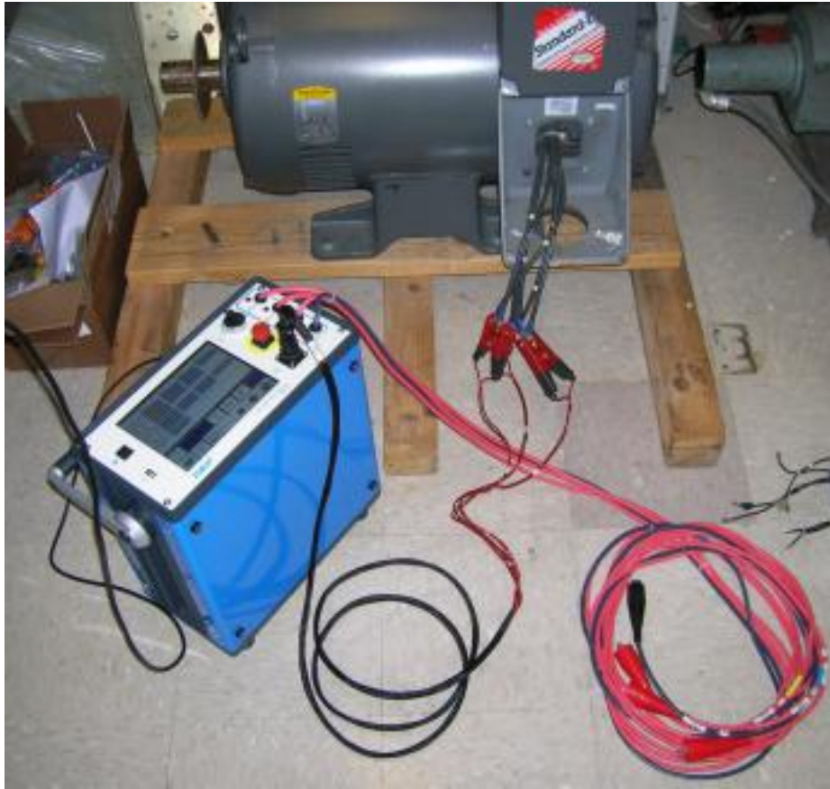
Figure 6. Baker DX connected to large motor with low-voltage test connectors for RLC testing; high-voltage connectors in foreground.
