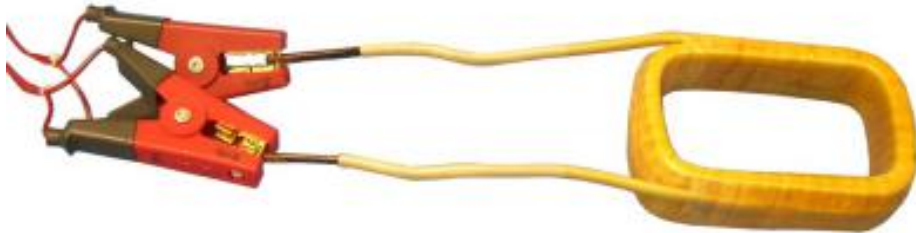
Figure 67. Connecting low-voltage cables to a coil.
