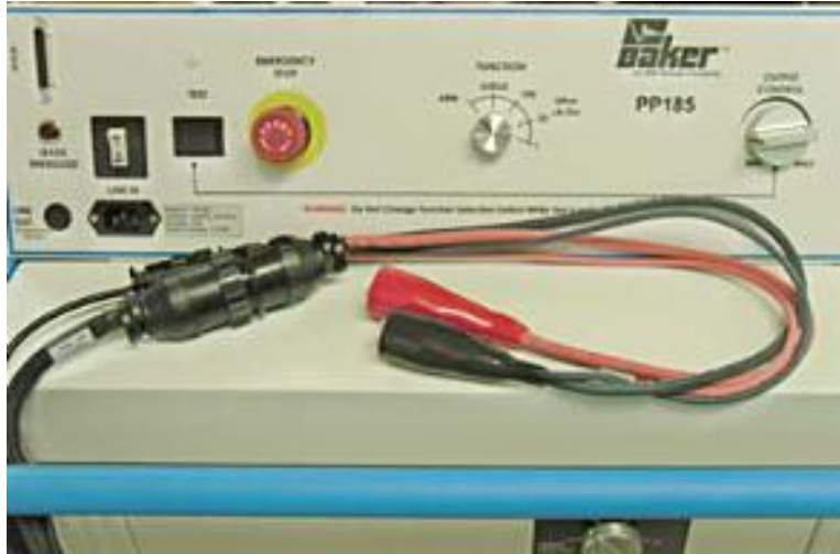
Figure 65. Connect test lead cable to clip accessory.
