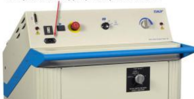
Figure 51. Connect power pack to AC source.
