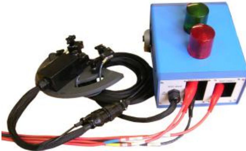
Figure 60. Baker ZTX connected to armature test fixture.
