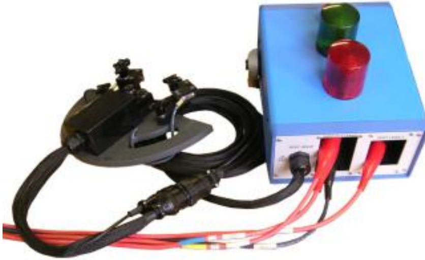
Figure 61. Baker ZTX with bar-to-bar armature test fixture.
