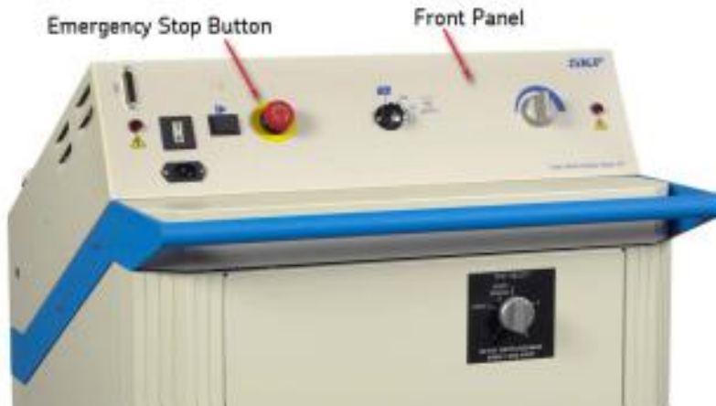
Figure 3. Power pack showing Emergency Stop button.
