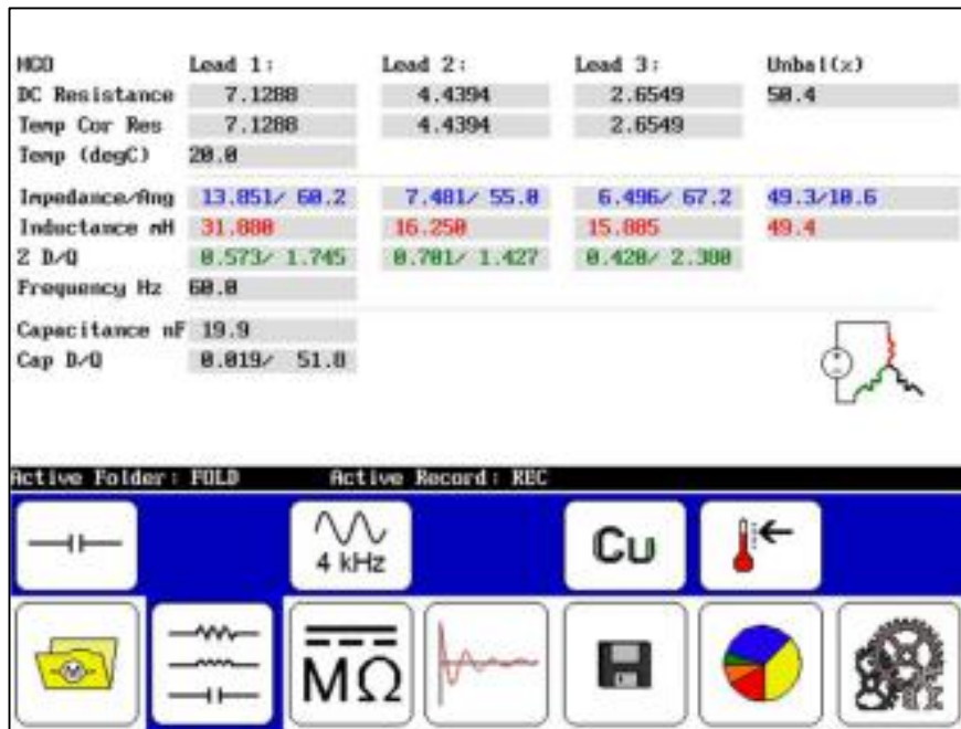
Figure 191. Completed RLC test screen.
