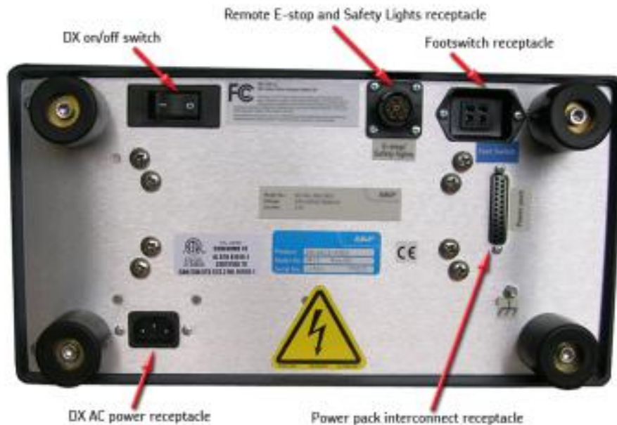
Figure 8. Rear panel connections.
