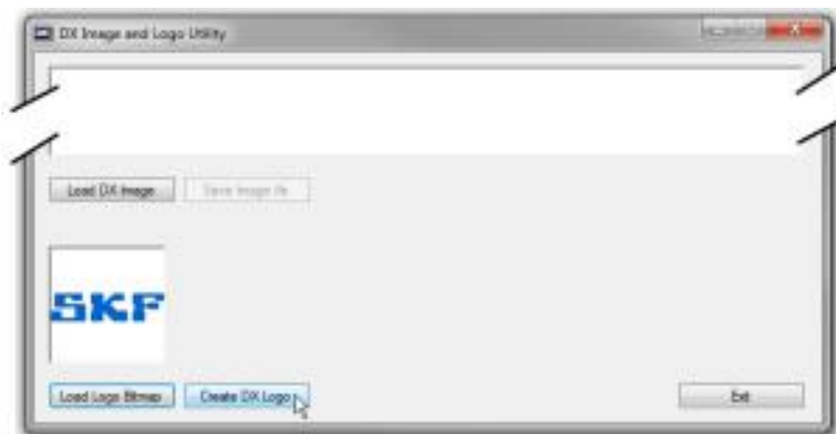
Figure 38. Using DX Utility software to load logo bitmap.
