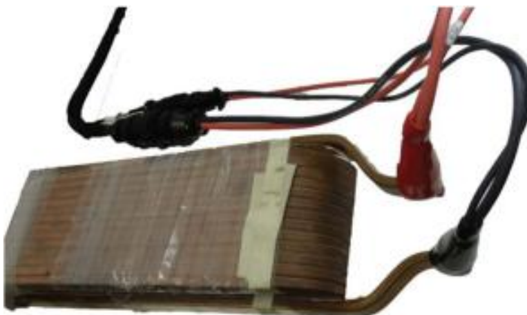
Figure 66. Connect clips accessory to DC interpole coil.
