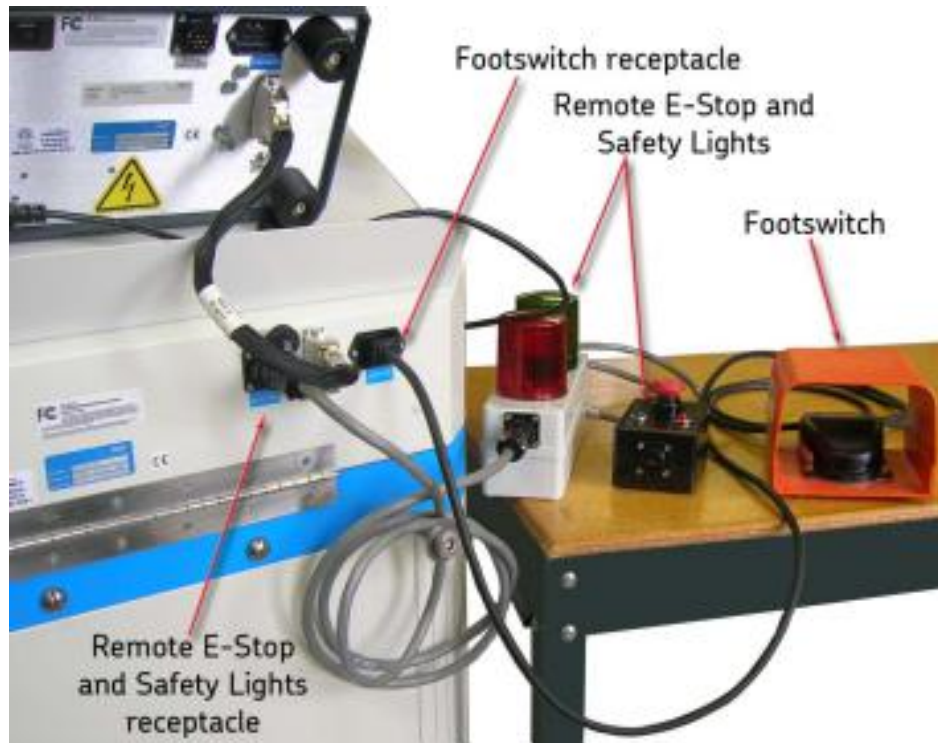
Figure 50. Attaching accessories to the power pack.
