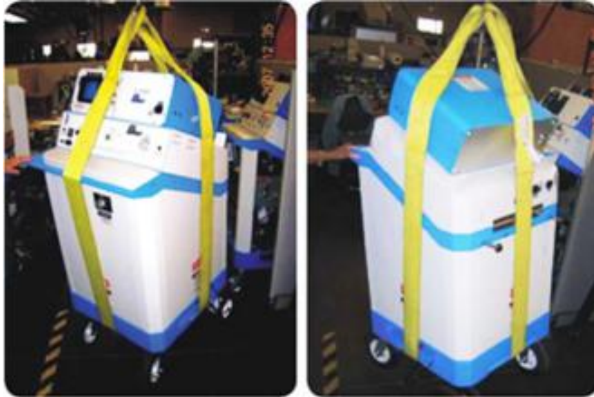
Figure 5. Properly lifting the unit using straps.
