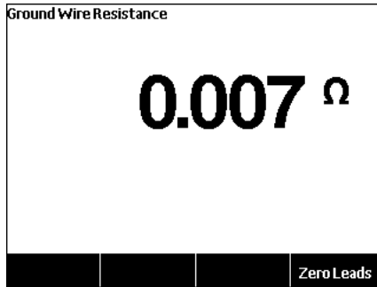
Figure 11. DUT Ground Resistance Measurement
