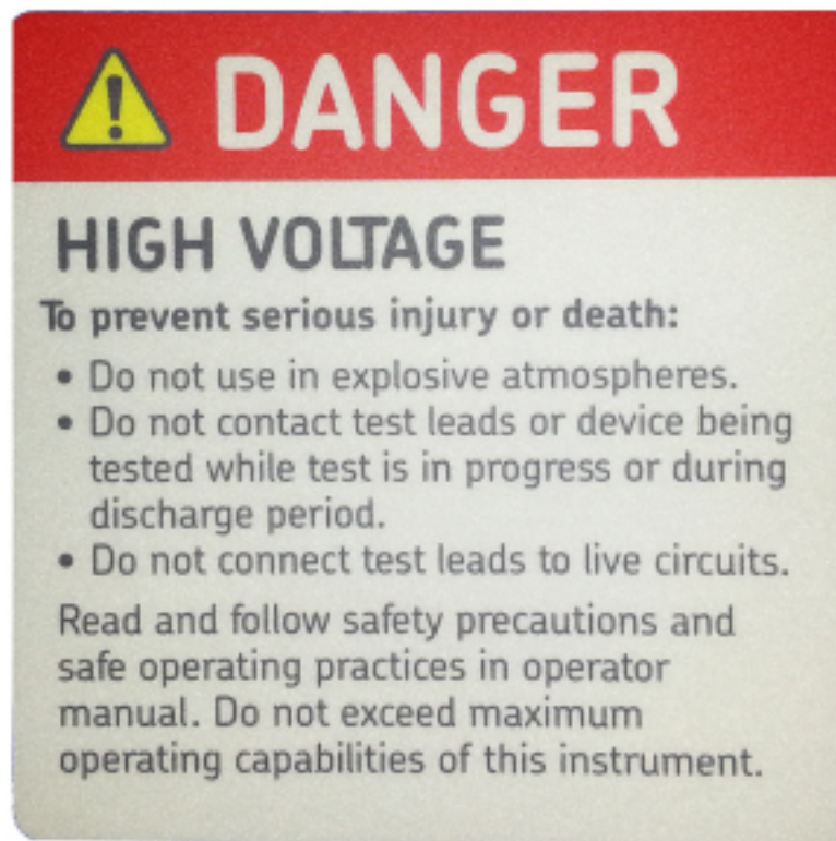
Figure 1. High voltage warning label.
